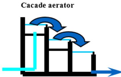
Figure 2. Illustration of Cascade technique
