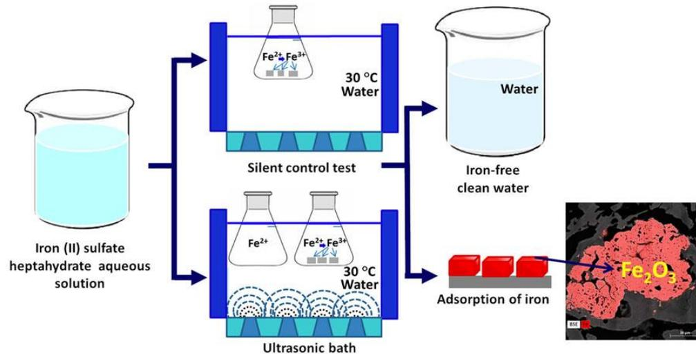
Figure 6. Illustration of Adsorption with ultrasound technic [6].
