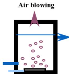
Figure 3. Illustration of Air blowing technique
